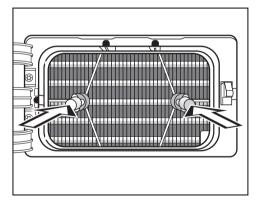
■ First insert the handle with the filter attached over the two guide pins.
